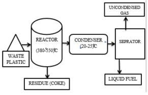
Figure: - 1 PYROLYSIS PROCESS
