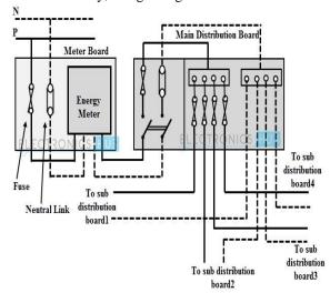
FIG. Electrical scheme of the main board
