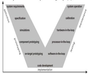
V-diagram of an embedded system design flow
