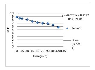
3. First order reaction for COD removal for Graphite Electrode.
