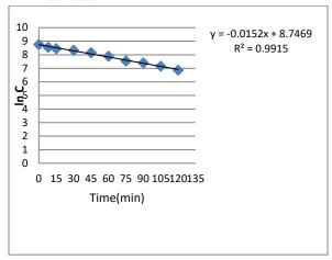
4. Second order reaction for COD removal for Graphite Electrode.
