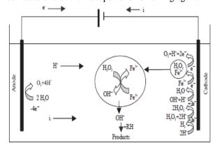
Fig 1: Schematic representation of reaction mechanism of Electro-Fenton process
