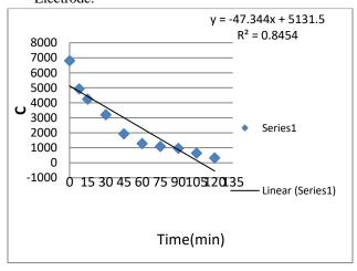
2. First order reaction for COD removal for Iron Electrode
