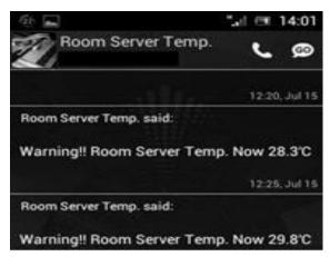
Fig 5: Message when temperature  $> 28^{\circ}$ C
