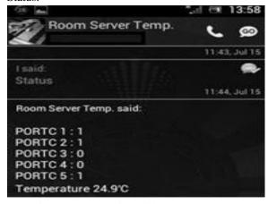
Fig 4: System testing with Status command
