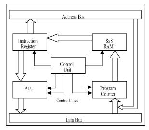
Figure.2. Controller Block Diagram
