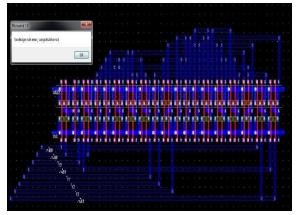
Fig 4.5.1: Layout Design of 2 - bit Multiplier. So in above we can see that layout design of the 2 - Bit Multiplier and it's DRC (Design Rule Check) was verified on Microwind spice tool. It's area is 53.8  $\mu$ m<sup>2</sup>.
