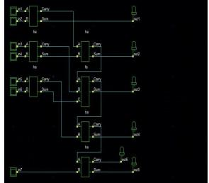
Fig 4.3: Schematic Design of Carry Save Adder 2
