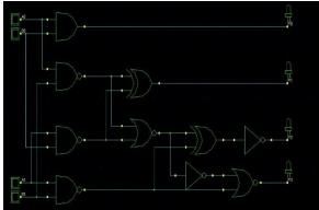
Fig 4.1: Schematic Designing of 2 - Bit Multiplier. The 4  $\times$  4 multiplication is done considering the grouping 2 bits together each of the 4 – Bit input.
