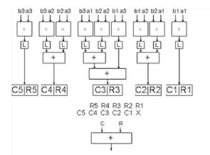
In this architecture pipeline approach has been implemented and latches have been used. Latches are used to stabilize the initial state.
