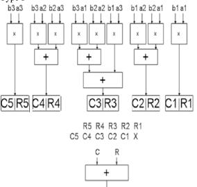
In this architecture 9 multipliers each of 4 bits, 4 adders of 8bits and 9 bits are used respectively
