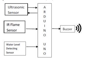
Fig 2: Working flow diagram of the proposed smart stick for blind system
