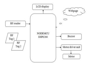
Figure 1 Block Diagram of Proposed Toll Gate System
