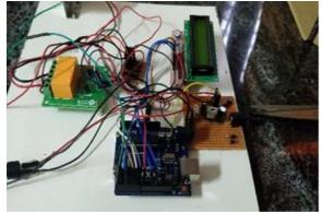
Figure 3 Toll unit- Hardware model The hardware model of RFID based toll unit system is shown in Figure 3, it consists of Ardunio uno, RFID Reader and Bridge driver
