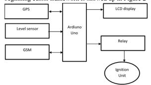
Figure 2 block diagram of GSM based vehicle theft
