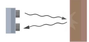
Figure 4 Diagram of the basic ultrasonic sensor operation
