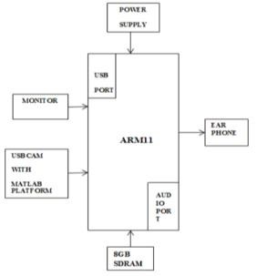
Figure 2 Block Diagram of Proposed System
