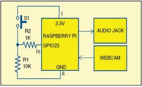
Figure. 6: Circuit connection to Raspi board
