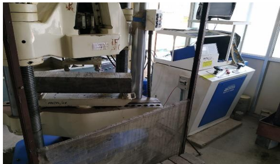
Figure 3.8 (a) and (b) Flexural strength test of Specimens
