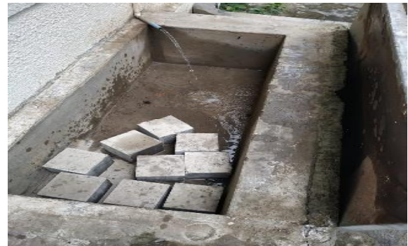
Figure 3.6 Curing of Specimens for Analysis
