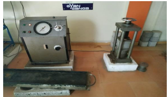
Figure 3.7 Crushing strength test of Specimens
