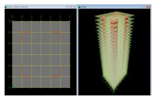
Fig.2- shear wall at interior of structure
