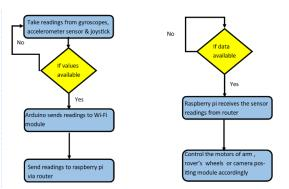
Fig.2,3 flow chart at operator and rover side
