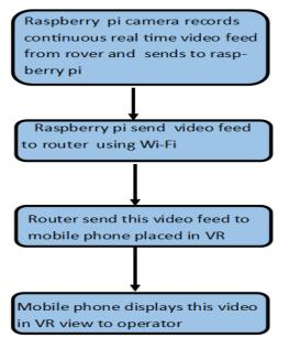
Fig.4 flow chart of operation of video streaming
