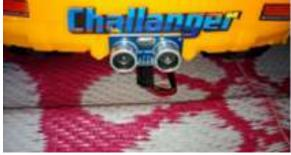
Fig 6: Ultrasonic Sensor C. Motor Driver (L293D)
