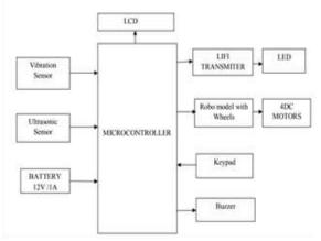
Fig 3: Transmitter Block Diagram
