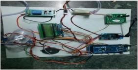
The hardware a part of the system has the sensors which are attached to the mask. The oxygen tank is going to be given through the motor to the mask. Using an adapter and an influence supply the facility is given to the circuit. Relay circuit is employed for the motor. Wi-Fi module will update details to the online page and the LCD display will display the conditions of the sensors.
