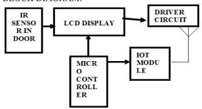
Fig. 1 Block Diagram of hardware Section
