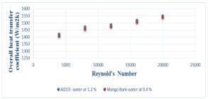
Figure 5. Comparison of overall heat transfer coefficient for (Al2O3)-water and Mango bark-water nano fluids at 1.2 % volume fraction
