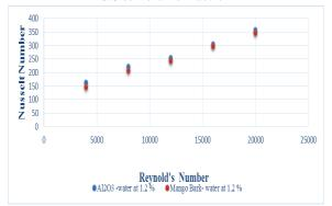
Figure 8. Comparison of Nusselt number for (Al2O3)-water and Mango bark-water nano fluids at 1.2 % volume fraction
