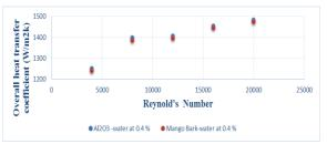
Figure 3. Comparison of overall heat transfer coefficient for (Al2O3)-water and Mango bark-water nano fluids at 0.4 % volume fraction
