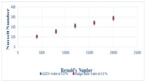
Figure 7. Comparison of Nusselt number for (Al2O3)-water and Mango bark-water nano fluids at 0.8 % volume fraction
