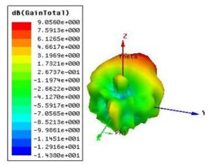
Figure 3.3: Total Gain of this Antenna
