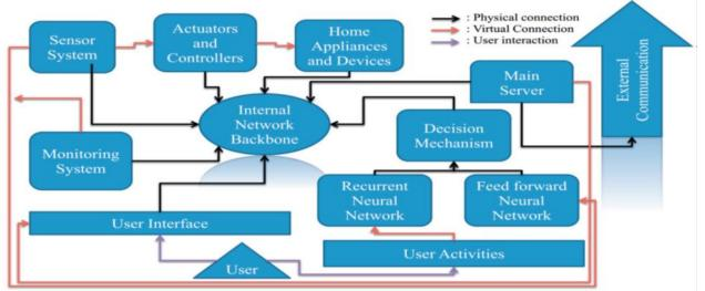
Fig.1 System Design Diagram
