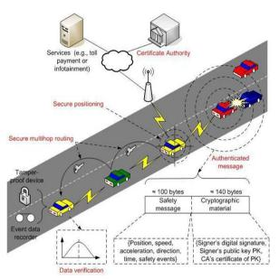
Figure 1.2 VANET Application Architecture
