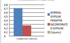
Fig.5. Compression strength comparison graph From the graph, it is concluded that normal gypsum cube has more compression strength than paraffin incorporated cube.
