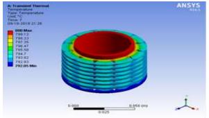
Fig 8 Temperature contour of cylindrical block having Magnesium alloy circular fin with triangular
