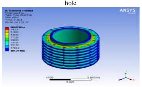
Fig 9 Total Heat flux contour of cylindrical block having Magnesium alloy circular fin with triangular hole
