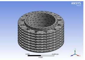
Fig 3 The meshing of cylindrical block having circular fins with triangular holes.
