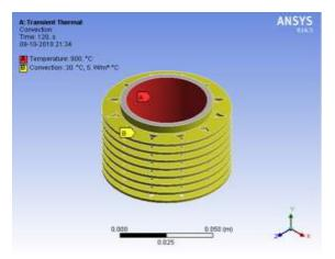
Fig 4 The Named selection of cylindrical block having circular fins with triangular holes.
