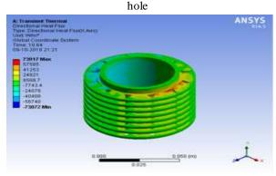
Fig 7 Directional heat flux contour of cylindrical block having Aluminium alloy circular fin with triangular hole
