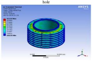
Fig 6 Total heat flux contour of cylindrical block having Aluminium alloy circular fin with triangular
