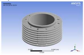
Fig 2 Geometry of cylindrical block having circular fins with triangular holes.
