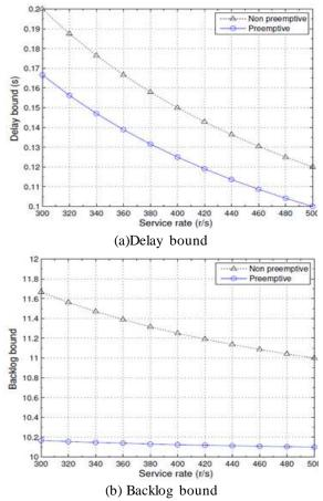
Fig. 4: Delay bound and backlog bound of fh with respect to preemptive scheduling and non-preemptive scheduling.
