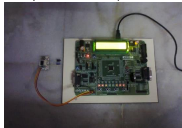
Fig4: Gas sensor interfacing with Arm 7
