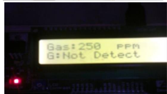
Fig4: Gas sensor interfacing with Arm 7
