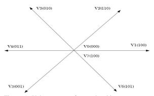
Figure 5: Voltage vector for two level inverter Look up table for voltage switching selection of two level inverter in Table 1. For every sector, selection of voltage vector is dependent on increment and decrement of torque and flux which is comes at output of hysteresis controller.
