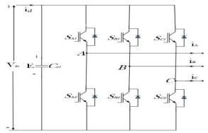
Figure 4: Circuit diagram of two level voltage source inverter
