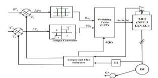
Figure 6: Block diagram of 3 level DTC technique Zero voltage vectors (zero magnitude)- V0 Small voltage vectors (0. 33 Vdc magnitude)- V1-V6 Medium voltage vectors (0.57 Vdc magnitude)- V6-V12
