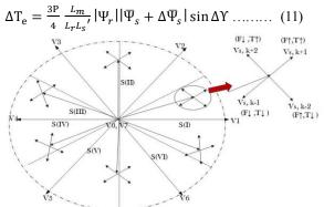
Figure 3: Selection of voltage vectors at changes in flux and torque [5]
