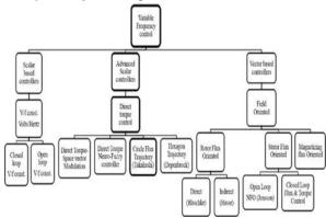
Figure 1: Types of speed control methods of an Induction motor
