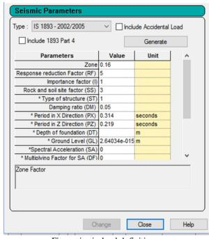
Fig: seismic load definition
