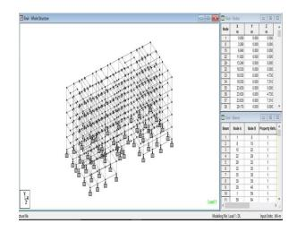
GENERATION OF THE STRUCTURE: The structure may be generated from the input file or mentioning the co-ordinates in the GUI. The figure below shows the GUI generation method.
