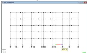
The Plan of G+4 was created by creating nodes on the x-z plane and the nodes are joined by using add beam tool
