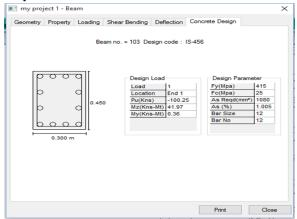
Fig: Concrete design of column no.103
