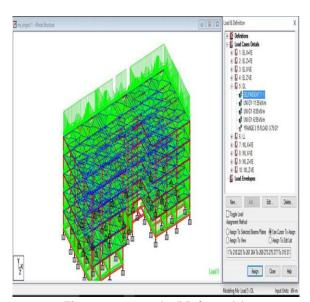
Fig: structure under DL from slab
