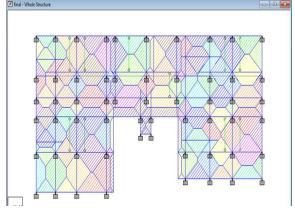
Fig: Dead floor load distribution
