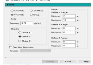
Fig: Input window of floor load generator
