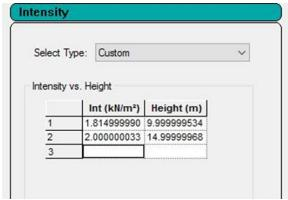
Fig: Design wind pressure at various heights
