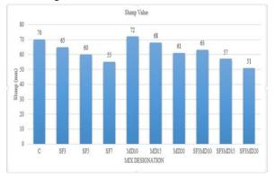
Figure no: 3 Response trace plot of Slump value. In this figure.3 is shows the slump value of concrete. The is same mix design. The slump value is measuring with the slump cone apparatus. In this figure different slump values are indicated in mm.
