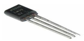
Fig.2 LM35 Temperature sensor
