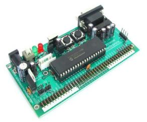
Fig.5 PIC Micro Controller
