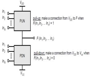
Fig. 1.0 - Pull-up and Pull-down network These fundamental approach works basically on two logics i.e. NAND and NOR logic,
