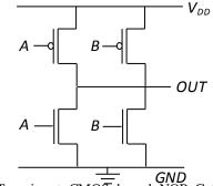
Fig. 3.0 Two input CMOS based NOR Gate using Parallel transistors combination
