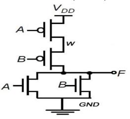
Fig. 2.0 - Two input CMOS based NOR Gate
