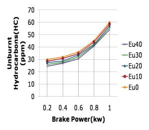
Fig. 8 Unburnt Hydrocarbons Vs Brake Power
