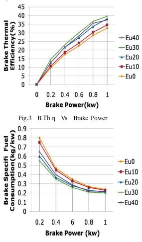
Fig.4 Bsfc Vs Brake Power
