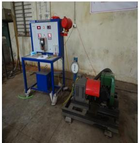
Fig.2 Experimental Setup Torque = Load (kg) x Arm Length (mm)
