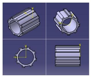
Sleeve with fine surface finish is showed in the figure above Material: Cast iron
