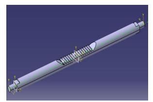
Rack with diameter 25 mm is shown in the figure above. At the ends of the rack threads were made for assembling the rack with tie rods. The surface finish needed is very fine for the rack to easily slide in the casing, so accordingly rack surface finish was achieved.
