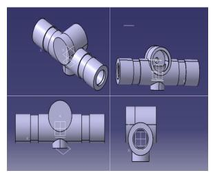
On both side of the casing grooves were made for mounting the casing into the chassis with the help of clamps.
