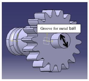
The extended portion which is shaft like is grooved at the centre for a steel ball to allow roll as shown in the fig which is to ensure minimum friction and to avoid wear and tear of the pinion.
