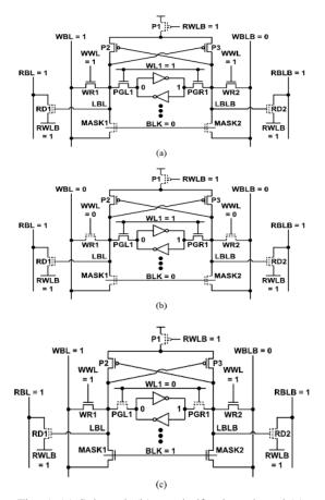
Fig. 5. (a) Selected, (b) row half-selected, and (c) column half-selected blocks of proposed SRAM architecture during write operation
