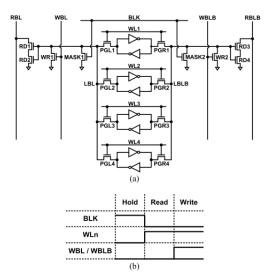
Fig. 2. (a) Average-8T SRAM architecture and (b) its operational waveform
