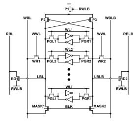
Fig. 3. Proposed SRAM architecture that stores i bits in one block
