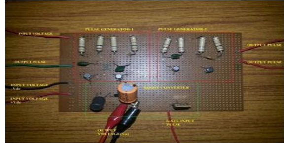
Fig.9. Open Loop DC to DC Boost converter kit A. Pulse Generator Part
