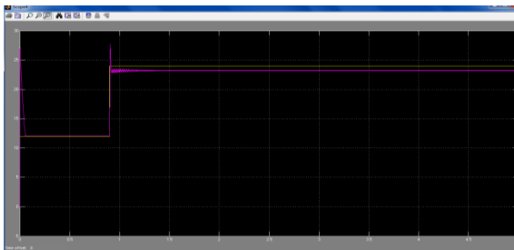
Fig.7. Simulated output voltage waveforms Simulation input voltage is 100V and output voltage is 200V and step voltage is 400V
