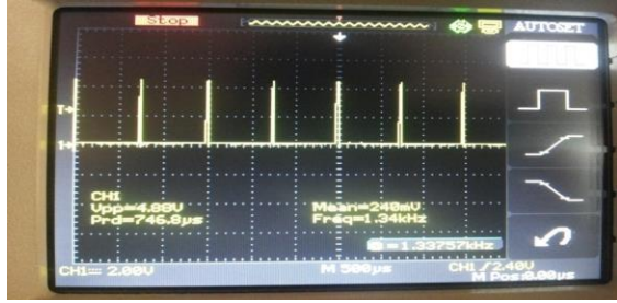
Fig.12 .Kit Response of gate pulse when T_{on} < T_{off}
