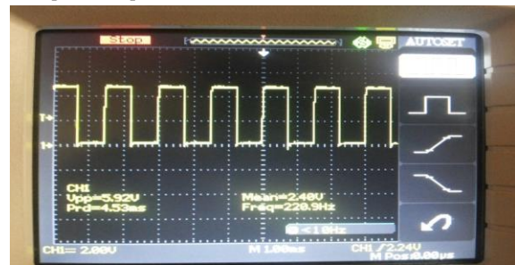
Fig.10. Kit Response of gate pulse when T_{on}=T_{off}
