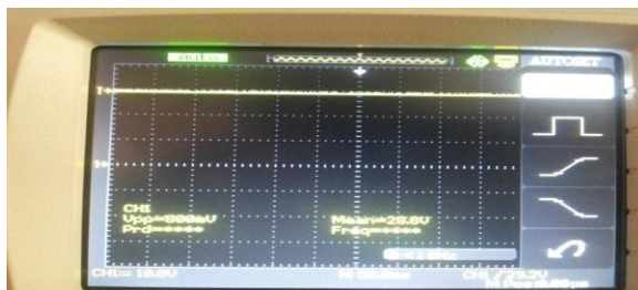
Fig.16. Kit Output Voltage 28.8V when Input voltage is 10V
