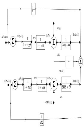
Load frequency control of two area system SIMULATION
