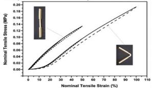
*Rubber-like SMH* (in original and pre-bent shapes) under cyclic loading at room temperature (about 22°C) and at high loading speed.
