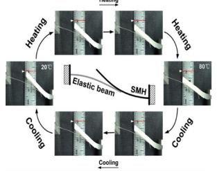
Two-way SME. Upon heating (top half, from left to right), the SMH beam pushes down the elastic beam (see inset for the illustration of set-up). Subsequently, upon cooling (bottom half, from right to left), the elastic beam pushes the SMH beam upward.
