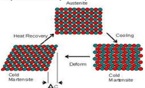
Microscopic and Macroscopic Views of the Two Phases of Shape Memory Alloys:
