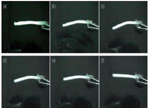
Triple-SME. Upon immersing into hot water, the SMH beam bends downward and then upward. Heating
