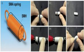
Self-healing of SMH. (a) SMH with an embedded SMA spring inside (illustration); (b1-b2) pulling SMH till fracture; (b3-b4) joule heating SMA coil for self-healing; (c) healed sample; (d) healed sample in bending.
