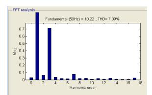
Fig 3. FFT spectrum for stator current of a 5-level inverter output
