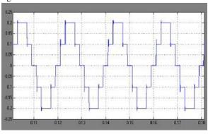
Fig 2. Experimental waveforms for stator current of a 5-level inverter output
