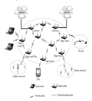
Fig.1.1 A Typical Infrastructure Wireless Mesh Network
