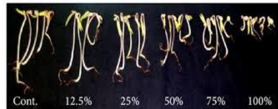
Figure 1: Effect of pulp and paper mill effluent (with dilution) on seedling growth
