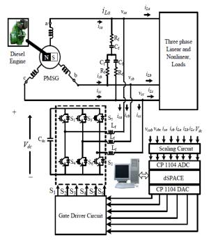
Fig. Configuration of PMSG based DG set feeding three phase loads.
