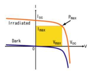
Schematic drawing of current-voltage characteristics of solar cell area of the yellow rectangle gives output power. Pmax denotes the maximum power point
