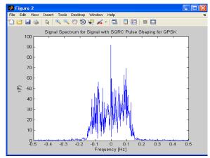
Fig .5 Spectrum of Square root raised cosine filter with  $\mathbf{OPSK}$
