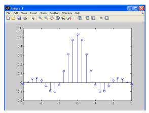
Fig. 2 coefficients of Square root raised cosine filter
