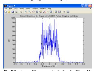
Fig .7 Spectrum of Square root raised cosine filter with  $$\mbox{8QAM}$$
