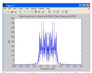
Fig .3 Spectrum of Square root raised cosine filter with BPSK
