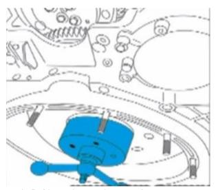
**Fig 5: Oil seal installation tool of Volvo Truck** 4. Large Scale Production of Small Engines: At the Large Scale industries of Motorbikes like Honda, Hero, Suzuki, etc. the Oil seals are installed with the help of electric screw type linear actuators. It generates sufficient torque and this is one of the fast ways of installation of oil seal.
