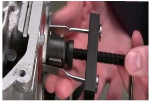
Fig 3: Oil Seal Installation at Workshop2. Heavy Duty Engines:
