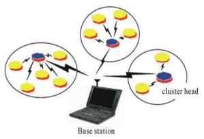
Figure 1: Clustering method in a sensor network
