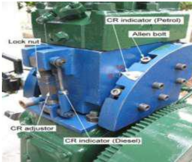
Fig.3 Compression ratio adjustment
