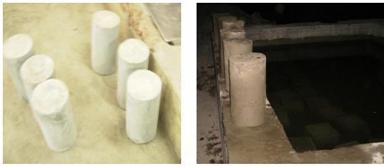
After removing from mould
