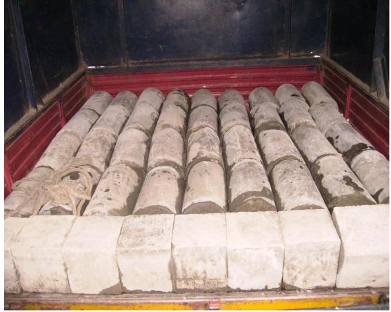
Carrying out 36 moulds to Durocrete Lab Compressive and Split tensile strength testing
