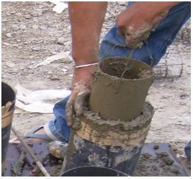
Removal of inner Mould
