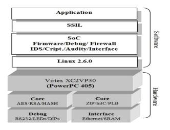
Figure 1. Hardware and Software of our Embedded System
