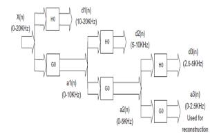
Fig: 1 An example of three level decomposition The equation to derive the high pass and low pass wavelet coefficients is given by:
