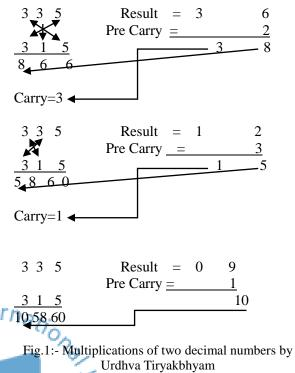
Algorithm for N x N bit Vedic multiplier Using Urdhva Tirvakbhyam for two binary numbers. For NxN multiplication, divided the multiplicand and multiplier into two parts, consisting of (N to N/2-1) bits and (N/2) bits. For example for multiplications of X and B, of 16 bits each, if X=0000001010101101 then its parts will be 00000010 and 10101101. Represent the above mentioned parts of X as Xm and XI. Similarly for the B, it is Bm and BL. Now can have
